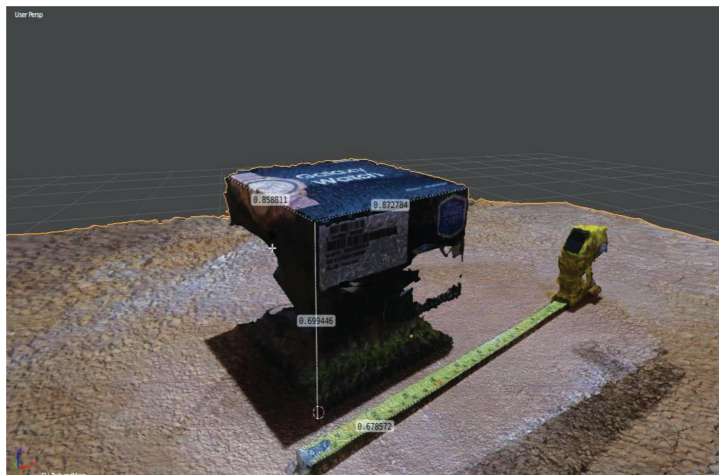
Figure 3. Box scanned using Photogrammetry with measuring tape as ground truth, rendered and measured in Blender
