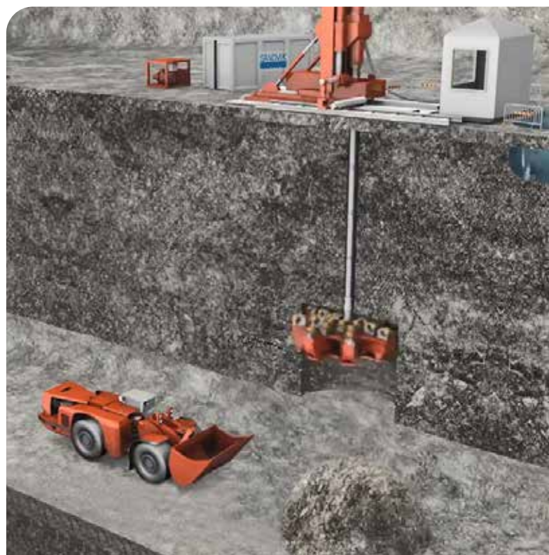
The raise boring rig works as follows: at first a hole is drilled from the ground surface into the underground part. Then an extension is attached to the cage, which the cage begins to pull back up. The diameter of the resulting bore hole is 3.1 meters.
