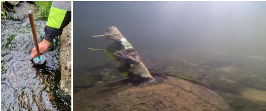
Figure 1. Hydromast device and an example of debris on the device
