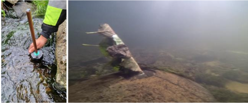
Figure 1. Hydromast device and an example of debris on the device
