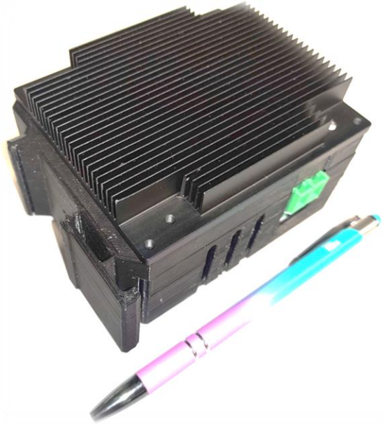
Smart DC SSCB (Safe Break) Short circuit fault isolation >10us
